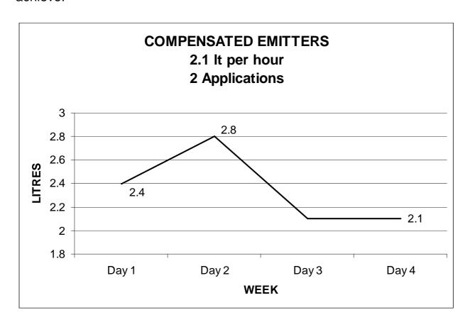
Some emitters become clogged by soft blockages in the open position thus delivering more water than it is designed to. During the 1 hour of treatment delivery may even increase before fowling is killed and flushed out of the emitters, when volume will decrease to the design specifications.
