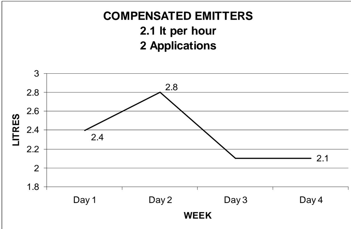
Some emitters become clogged by soft blockages in the open position thus delivering more water than it is designed to. During the 1 hour of treatment delivery may even increase before fouling is killed and flushed out of the emitters, when volume will decrease to the design specifications.
