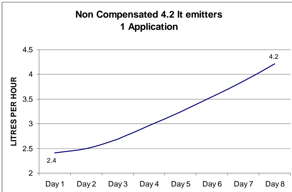
Emitters with a large delivery are much easier to clean than those with a small delivery. It is necessary to use the water flow to remove the treated bacteria; this in severe cases may take a few days and a number of irrigation cycles to achieve.
